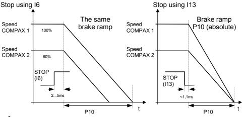
Using I13 for stop bring both axes to a stop simultaneously.
